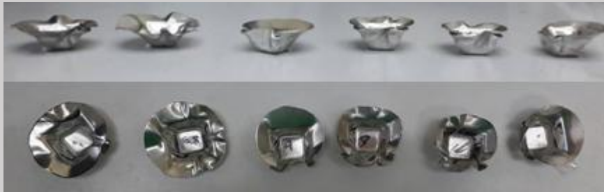
Figure 2. Square deep drawn part with various defect can be observed.
