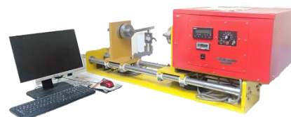
Twist forming machine utilized by FYP and Master students after minor repair and add load a cell.
