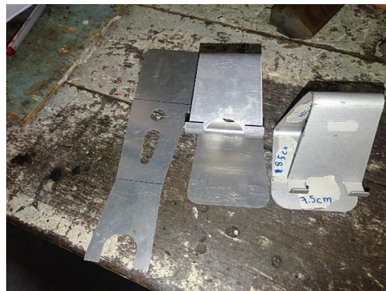
Before and after bending part, compared to reference product.
